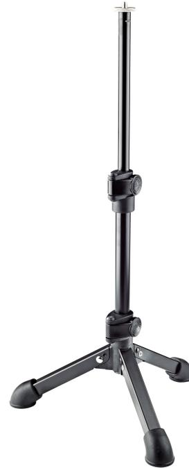
The telescopic microphone stand with a 1/4" threaded connector is extremely versatile. Its height can be adjusted from 230 to 400 mm using the practical clamping lever. This light-weight three-legged stand with folding legs is suitable for mobile operation. The robust foot end caps provide stability and reduce undesirable transmission noise.
